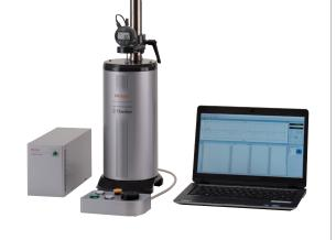
Mitutoyo's I-Checker achieves the highest accuracy in its class and can guarantee ultra-reliable inspection results. This instrument can be connected to your laptop using a USB cable and has a control box for ease of operation.
